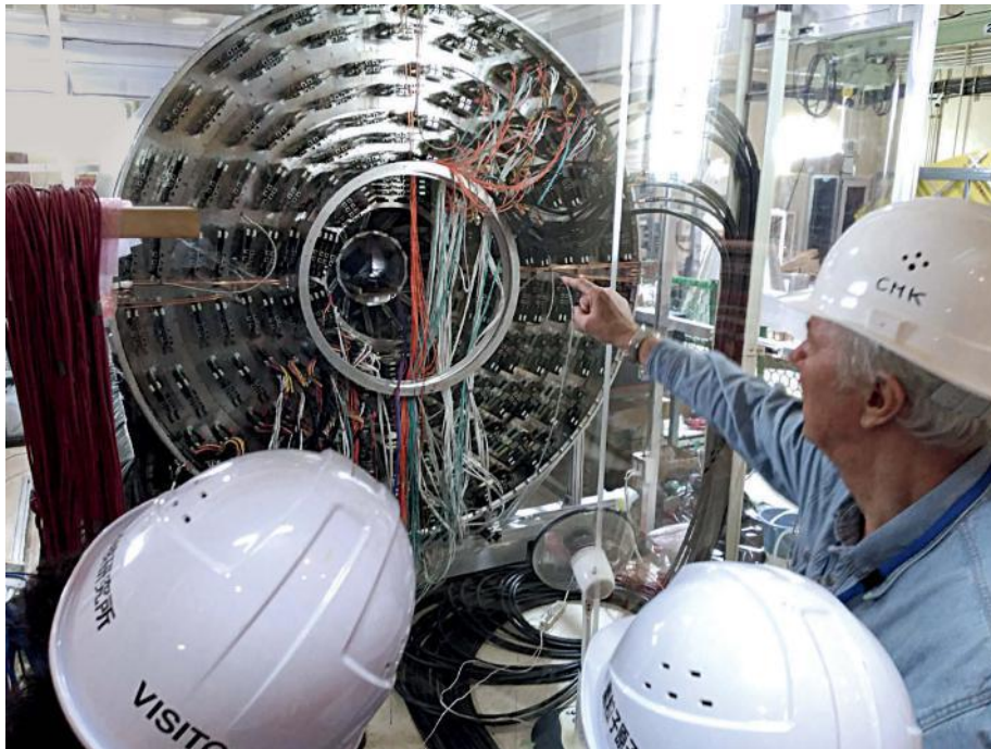
Christian Kiesling (right) and his colleagues assess the progress as the Belle-II detector at SuperKekB is being set up. Kiesling points to an opening that will house the vertex detector, whose task is to determine the exact position of the decay. The heart of this instrument is the dual-layer pixel detector (top left), inside which the decays take place. It is composed of modules whose image sensors each comprise 200,000 pixels (bottom left).
